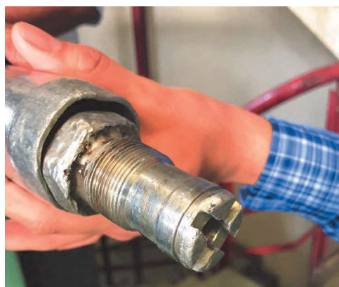
Damage to threads on SDX® III Nozzle.
