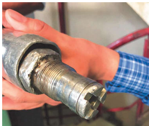
Damage to threads on SDX® III Nozzle.
